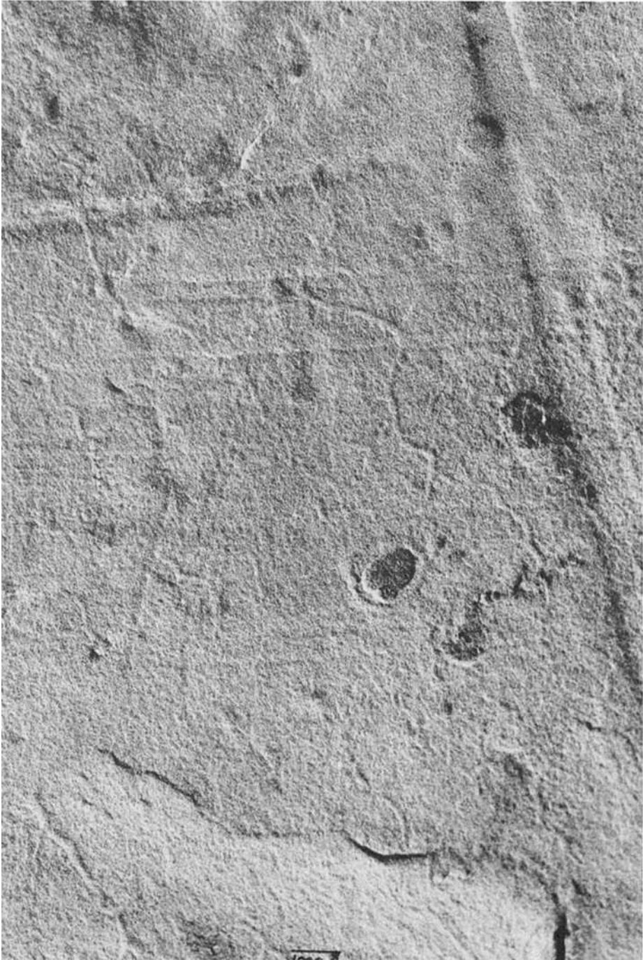
Fig. 2. Transmission electron micrograph of a surface replica of a polysulfone hollow fiber membrane.
